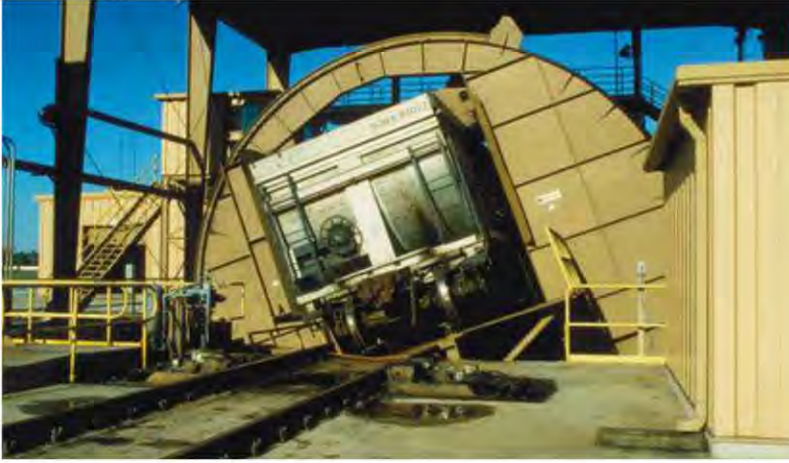
Rotary railcar dumper, manufactured by Heyl & Patterson.
