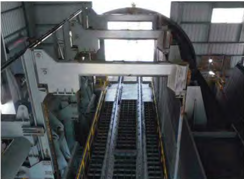
Heyl & Patterson's hybrid machine can dump coal like a rotary dumper and also receive bottom dump railcars.
