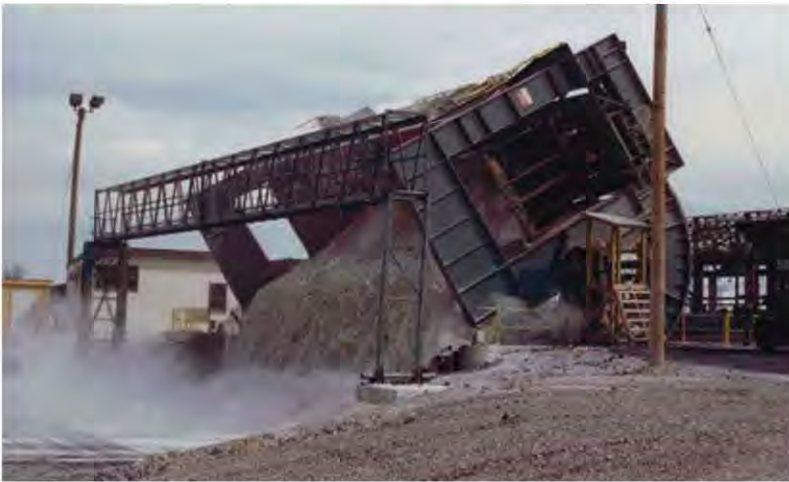
Heyl & Patterson turnover dumper similar to the one being installed in Argentina for Oxbow Carbon.
