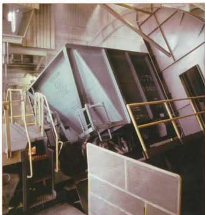
Railcar Dumpers come in a variety of designs including the 'Turnover', 'C shaped' or 'Rotary dumper' design.
